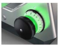
Green means motor off gauge plate closed.
